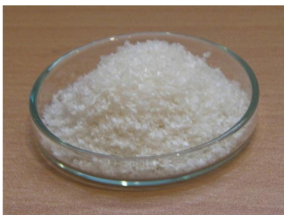
Fig.3. Prepared chitosan from shrimp shells in Nanomedicine and Tissue Engineering Research Center.
